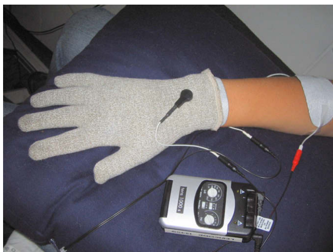
Fig. 1. Mesh-glove: a two-channel stimulator delivers a train of 50 Hz stimuli (pulse width 300 \mu s) with the amplitude above the threshold for sensation (ranging from 2.4 to 3.6 mA). The mesh-glove acts as a common anode, the cathodes are placed over the tendons of the forearm flexors and extensors.
